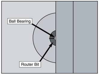
**Figure 23.** Proper setup for profile cutting. (Top View)
